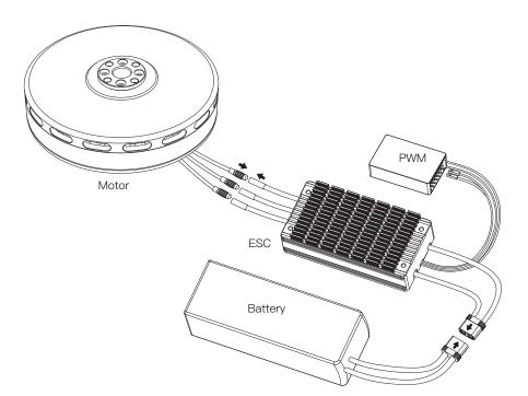
Black wire: ground wire White cable: throttle signal cable Yellow cable: error signal cable Orange cable: RPM signal cable RPM conversion formula:
