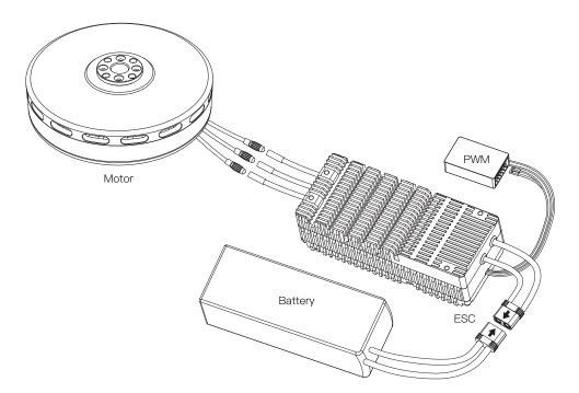
Black wire: ground wire White cable: throttle signal cable Yellow cable: error signal cable Orange cable: RPM signal cable RPM conversion formula:
